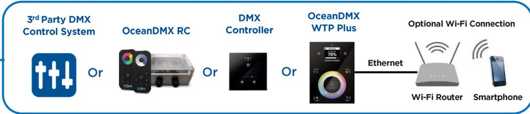
Details how to connect the DMX control device can be found in the product installation manual attached with the device.
